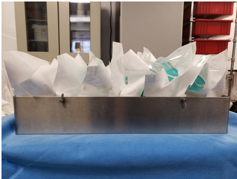
Figure 3: Up to twelve (12) individually packaged respirators placed side-by-side in a sterilization basket.
